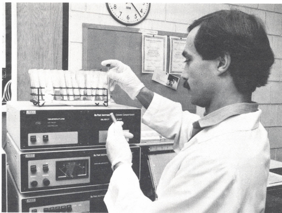
Paul Maniscalco, Senior Tech Chem, injects a serum sample into this instrument producing a graph from which the drug level can be determined. (A/V Photo)
